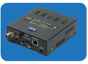
Configuration and status of the system can be done through the Ethernet interface using a Web browser, or through a command line using Telnet or SSH. An RS-232 I/O is also available for configuration and status using the command line interface. The Model 8461 can be powered from an external wall plug AC/DC power supply or from Power over Ethernet (PoE) capable switches.
